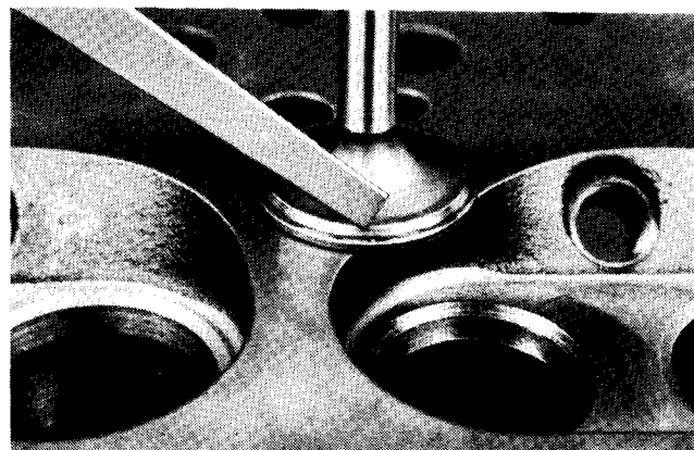
Checking for Proper Valve Seating
