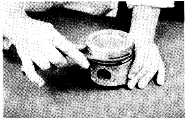
Checking Ring Clearance in Groove
