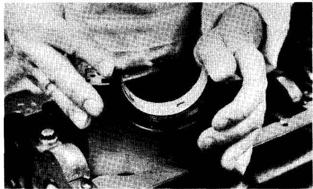
Rear Main Bearing Cap and Filler Block
